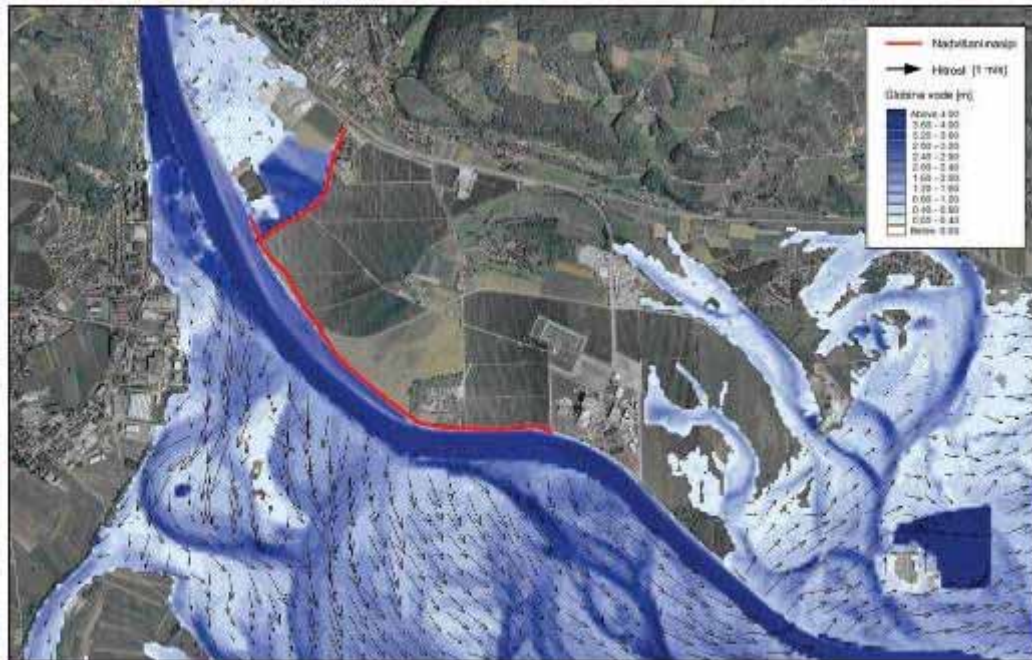
Figure 1: Flood protection of the Krško NPP for beyond basis flood (10,000 m 3 /s)
