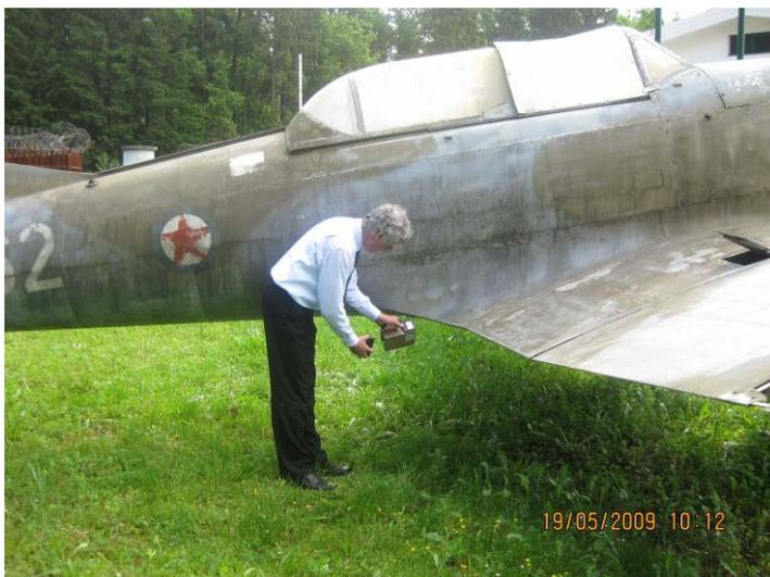
**Figure 13:** Airplane with altimeter containing a radioactive source above exemption level
