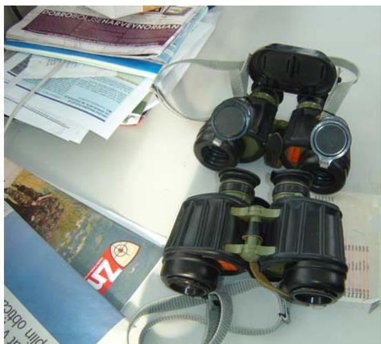
**Figure 12:** Binoculars with  $^3\text{H}$  of 37 GBq i.e. well above exemption level of 1 GBq
