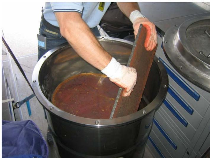
**Figure 15:** Packaging the radioactive source for a transport
