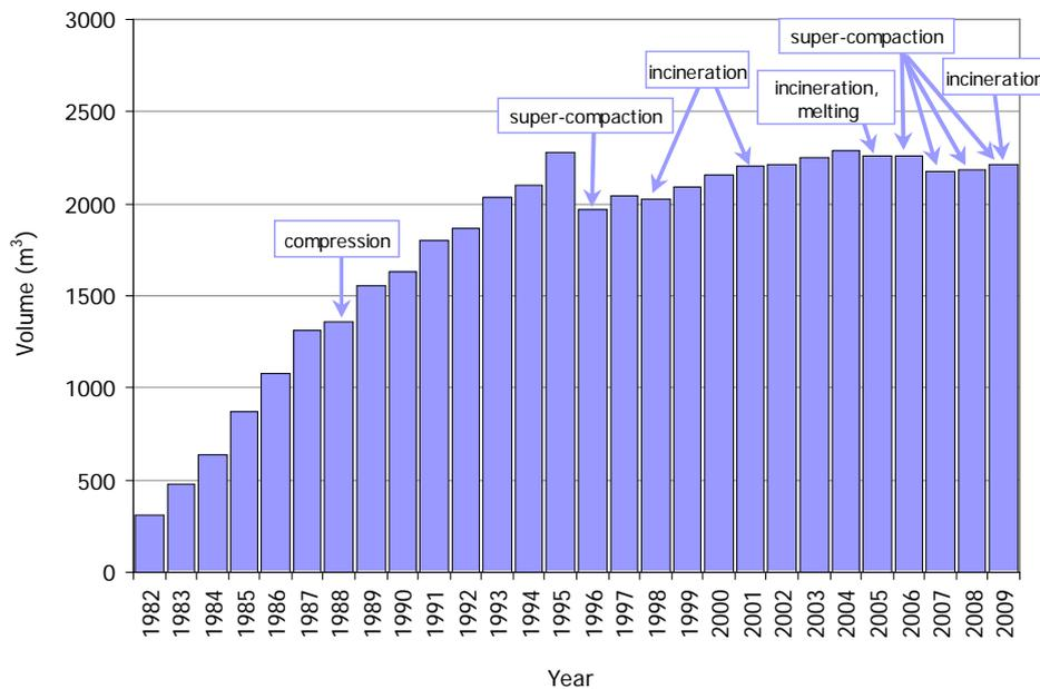
**Figure 20:** Accumulation of low and intermediate level radioactive waste at the storage in the Krško NPP
