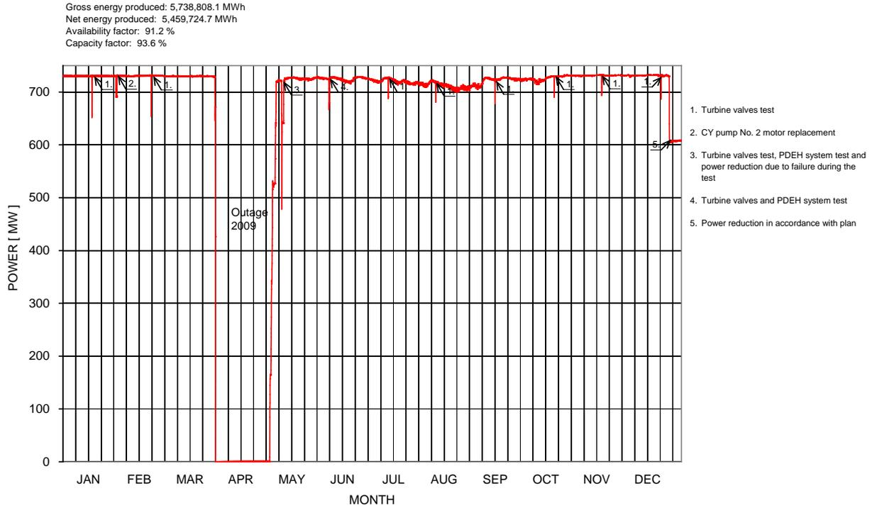
Figure 1: Operating power diagram for the Krško NPP in 2009
